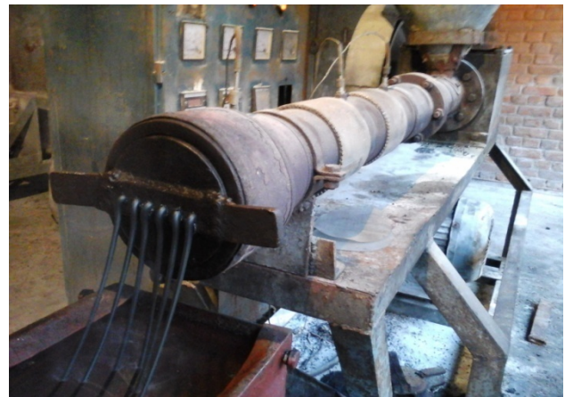
Fig. 1: Batch Mixing Extrusion Machine
